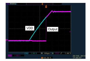
Figure 22. Output Behavior vs. Supply Voltage NCP81071A (Inverting) 10 nF between Output and GND, INA = GND, ENA = VDD
