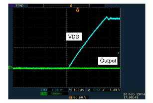
Figure 28. Output Behavior vs. Supply Voltage NCP81071B (Non-Inverting) 10 nF between Output and GND, INA = GND, ENA = VDD
