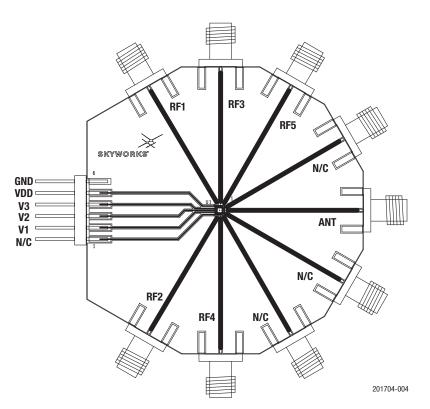
Figure 4. SKY13415-485LF Evaluation Board Assembly Diagram
