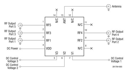
Figure 3. SKY13415-485LF Evaluation Board Schematic
