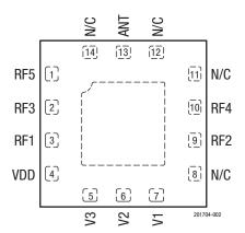
Figure 2. SKY13415-485LF Pinout (Top View)
