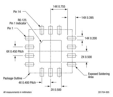
Figure 5. SKY13415-485LF PCB Layout Footprint (Top View)
