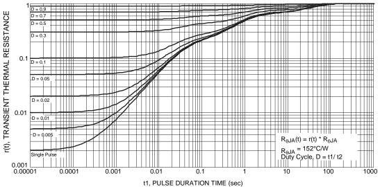
Figure 13 Transient Thermal Resistance
