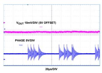
FIGURE 25. NON-SYNCHRONOUS BUCK, FORCE PWM MODE,  $V_{\text{IN}}$  12V, NO LOAD
