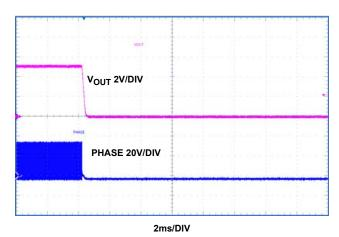
FIGURE 19. SYNCHRONOUS BUCK MODE, V<sub>IN</sub> 36V, I<sub>O</sub> 2A, ENABLE OFF
