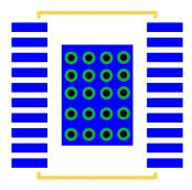
FIGURE 38. PCB VIA PATTERN
