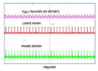
FIGURE 23. V<sub>IN</sub> 24V, 80mA LOAD, PFM MODE
