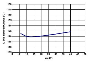
FIGURE 14. IC DIE TEMPERATURE UNDER +105 °C AMBIENT TEMPERATURE, 100 CFM, 500kHz,  $V_{OUT} = 5V$ ,  $I_{O} = 2A$
