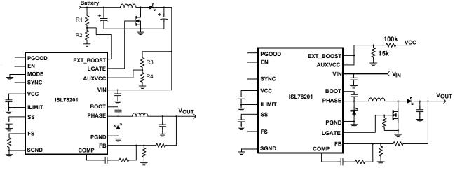
FIGURE 6A. 2-STAGE BOOST BUCK FIGURE 6B. NON-INVERTING SINGLE INDUCTOR BUCK BOOST FIGURE 6. BOOST-BUCK CONVERTER SCHEMATICS
