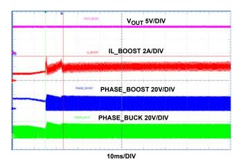
FIGURE 29. BOOST BUCK MODE,  $V_0 = 9V$ ,  $I_0 = 1.8A$ , BOOST INPUT DROPS FROM 16V TO 9V DC
