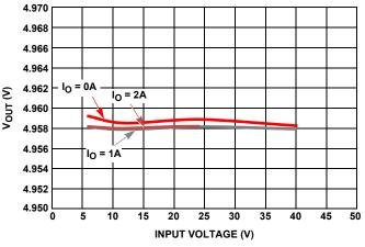
FIGURE 9. LINE REGULATION, V<sub>OUT</sub> 5V, T<sub>A</sub> = +25°C
