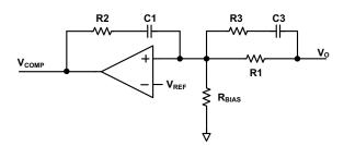
FIGURE 36. TYPE III COMPENSATOR
