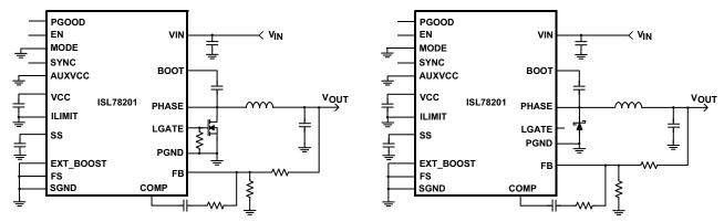
FIGURE 4A. SYNCHRONOUS BUCK FIGURE 4B. NON-SYNCHRONOUS BUCK FIGURE 4. SYNCHRONOUS AND NON-SYNCHRONOUS BUCK SCHEMATICS
