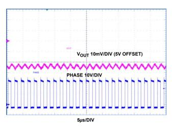
FIGURE 26. NON-SYNCHRONOUS BUCK, FORCE PWM MODE,  $\rm V_{IN}$  12V, 2A
