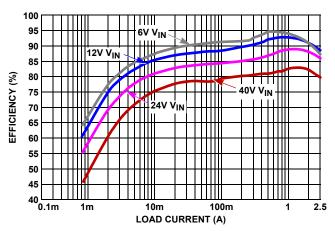
FIGURE 12. EFFICIENCY, SYNCHRONOUS BUCK, PFM MODE,  $V_{OUT}$  3.3V,  $T_A$  = +25  $^{\circ}$  C
