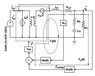
FIGURE 35. SMALL SIGNAL MODEL OF BUCK REGULATOR
