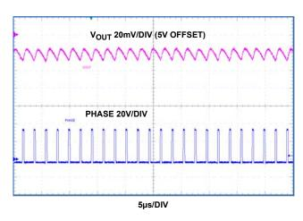
FIGURE 21. SYNCHRONOUS BUCK WITH FORCE PWM MODE,  $$V_{IN}$\,36V, I_{O}$\,2A$
