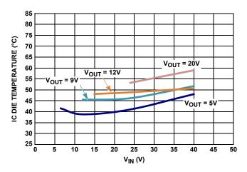
FIGURE 15. IC DIE TEMPERATURE UNDER +25°C AMBIENT TEMPERATURE, STILL AIR, 500kHz,  $I_0$  = 2A
