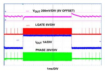
FIGURE 24. V<sub>IN</sub> 24V, 0 TO 2A STEP LOAD, PFM MODE
