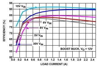
FIGURE 30. EFFICIENCY, BOOST BUCK, 500kHz, VOLIT 12V, TA = +25°C
