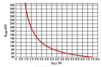
FIGURE 34. R<sub>LIM</sub> vs I<sub>OC1</sub>
