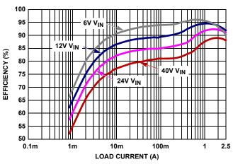
FIGURE 8. EFFICIENCY, SYNCHRONOUS BUCK, PFM MODE,  $V_{OUT}$  5V,  $T_A$  = +25°C
