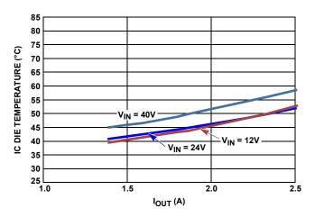
FIGURE 16. IC DIE TEMPERATURE UNDER +25°C AMBIENT TEMPERATURE, STILL AIR, 500kHz, V<sub>OUT</sub> = 9V
