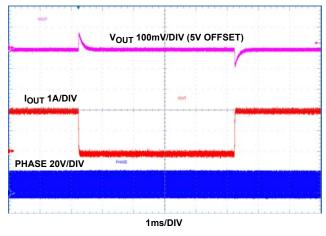
FIGURE 22.  $V_{\text{IN}}$  24V, 0 TO 2A STEP LOAD, FORCE PWM MODE
