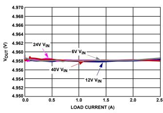
FIGURE 10. LOAD REGULATION, VOUT 5V, TA = +25°C
