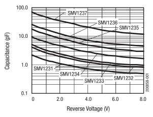
Figure 1. Capacitance vs Reverse Voltage
