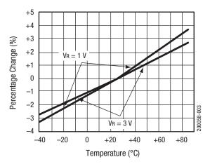
Figure 3. Relative Capacitance Change vs Temperature
