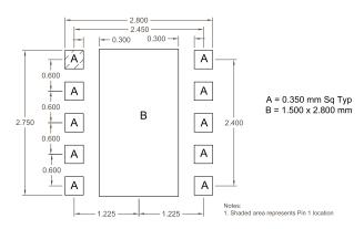
Figure 1. PCB Metal Land Pattern (Top View)
