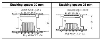
Note: The 🖂 in each model number are replaced with the number of contacts (16, 20, or 32). With 16 contacts, for example, the model number is XC5B-1631-3.
