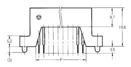
XC5K DIP terminal cross-section diagram
