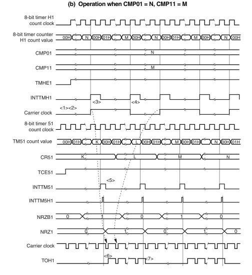
Figure 8-18. Carrier Generator Mode Operation Timing (2/3)
