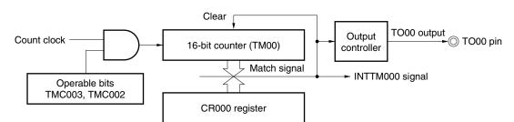
Figure 6-16. Block Diagram of Square-Wave Output Operation
