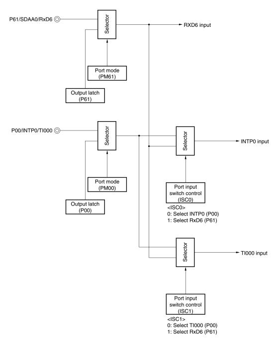
Remark ISC0, ISC1: Bits 0 and 1 of the input switch control register (ISC) (refer to Figure 14-11)
