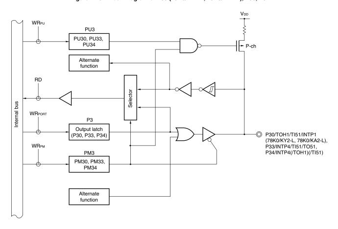
Figure 4-15. Block Diagram of P30 (78K0/KY2-L, 78K0/KA2-L), P33, P34
