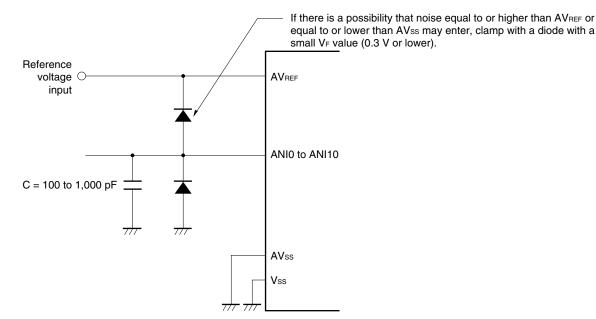
Figure 12-22. Analog Input Pin Connection
