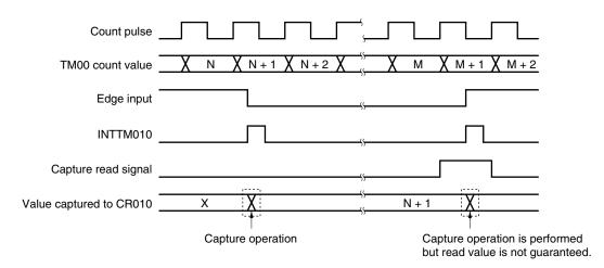
Figure 6-57. Timing of Holding Data by Capture Register
