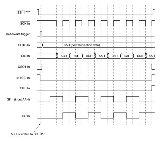
**Note** The SSE11 flag and SSI11 pin are available only for serial interface CSI11 of 78K0/KA2-L (25, 32-pin products) and 78K0/KC2-L (48-pin products), and are used in the slave mode.
