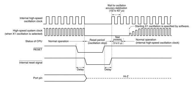
Figure 20-2. Timing of Reset by  $\overline{\text{RESET}}$  Input
