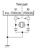
Figure 25-5. Example of Mounting Test Pads
