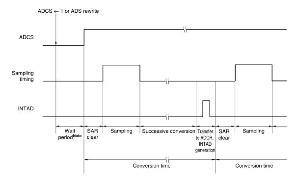
Figure 12-4. A/D Converter Sampling and A/D Conversion Timing
