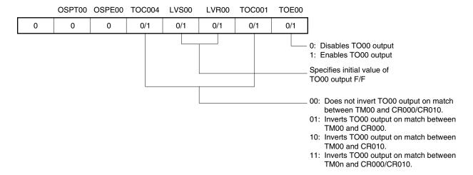
Figure 6-39. Example of Register Settings in Free-Running Timer Mode (2/2)
