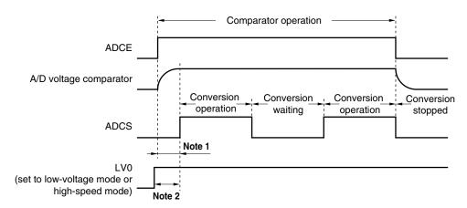
Figure 12-3. Timing Chart When Comparator Is Used
