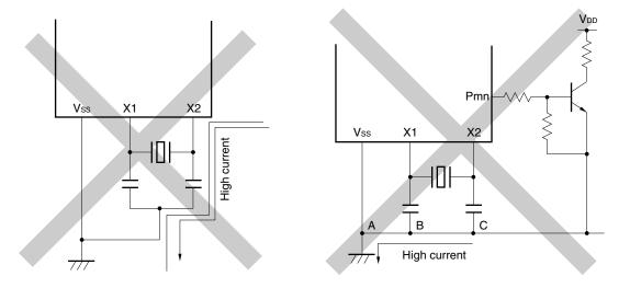
**Remark** When using the subsystem clock, replace X1 and X2 with XT1 and XT2, respectively. Also, insert resistors in series on the XT2 side.
