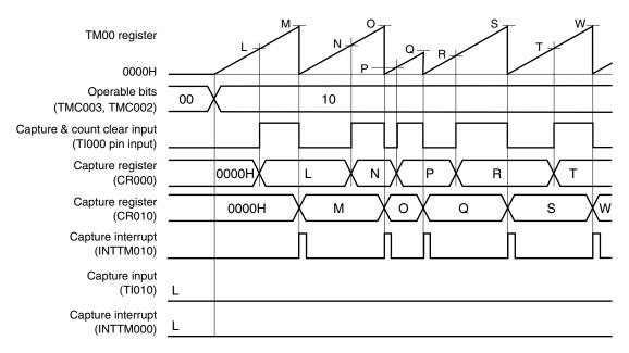
This is an application example where the pulse width of the signal input to the TI000 pin is measured.
