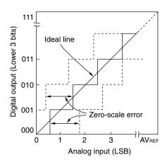
Figure 12-20. Integral Linearity Error
