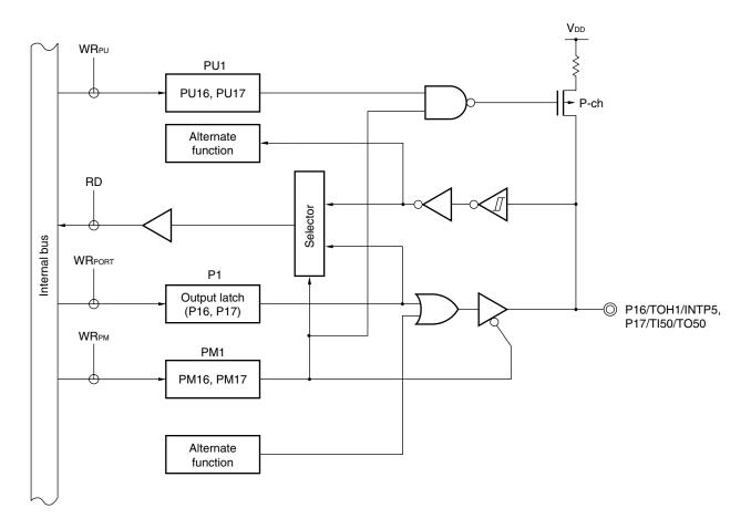
Figure 4-10. Block Diagram of P16 and P17
