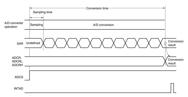
Figure 12-13. Basic Operation of A/D Converter
