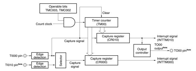
Note The timer output (TO00) cannot be used when detecting the valid edge of the Tl010 pin is used.
