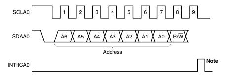
**Note** INTIICA0 is not issued if data other than a local address or extension code is received during slave device operation.
