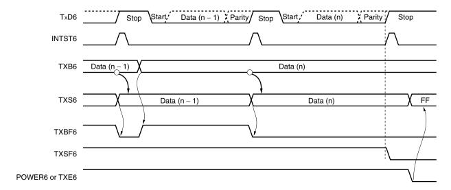
Figure 14-20. Timing of Ending Continuous Transmission
