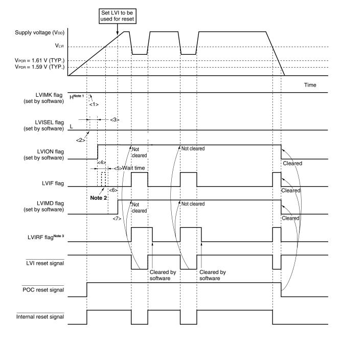
Figure 22-5. Timing of Low-Voltage Detector Internal Reset Signal Generation
