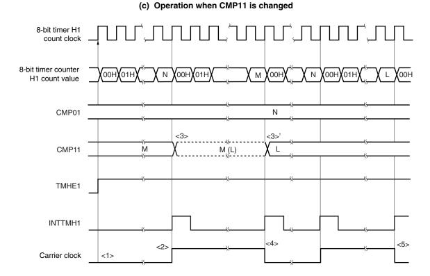
Figure 8-18. Carrier Generator Mode Operation Timing (3/3)
