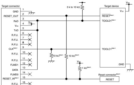
Figure 26-1. Connection Example of QB-MINI2 and 78K0/Kx2-L Microcontrollers (3/3)
