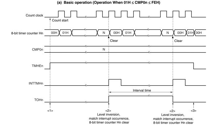
Figure 8-13. Timing of Interval Timer/Square-Wave Output Operation (1/2)
