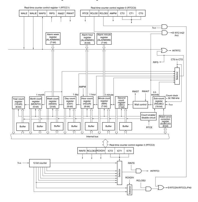
Figure 10-1. Block Diagram of Real-Time Counter
