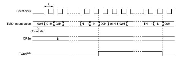
Figure 7-17. Square-Wave Output Operation Timing
