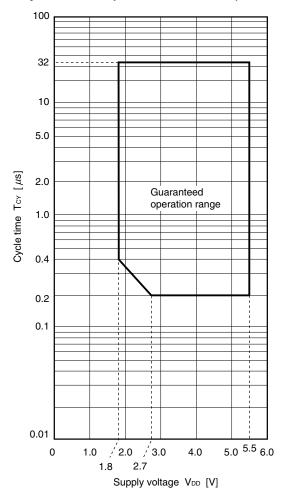
TCY VS. VDD (Main System Clock Operation, RMC = 56H (Low Power Consumption Mode))
