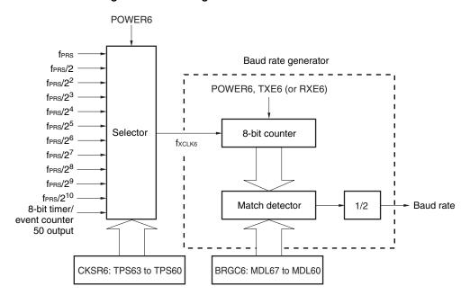
Figure 14-26. Configuration of Baud Rate Generator
