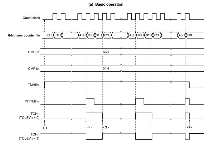
Figure 8-15. Operation Timing in PWM Output Mode (1/4)
