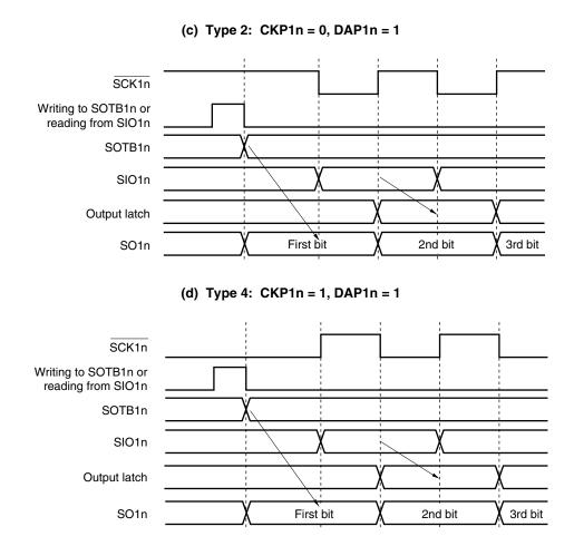
Figure 16-17. Output Operation of First Bit (2/2)
