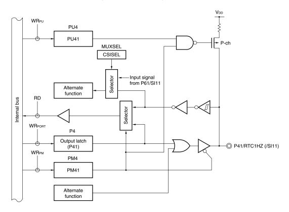
Figure 4-20. Block Diagram of P41
