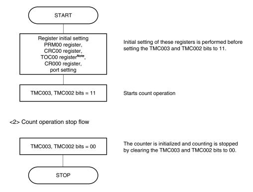
Note Care must be exercised when setting TOC00. For details, refer to 6.3 (3) 16-bit timer output control register 00 (TOC00).
