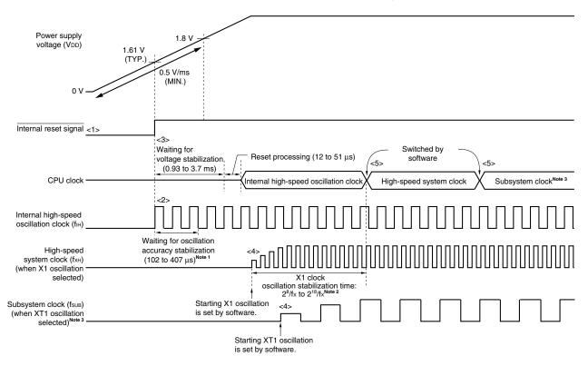
Figure 5-16. Clock Generator Operation When Power Supply Voltage Is Turned On (When LVI Default Start Function Stopped Is Set (Option Byte: LVISTART = 0))
