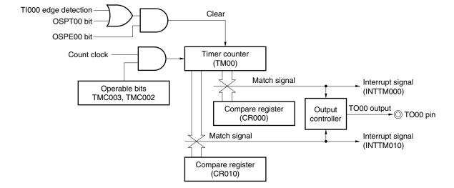
Figure 6-44. Block Diagram of One-Shot Pulse Output Operation
