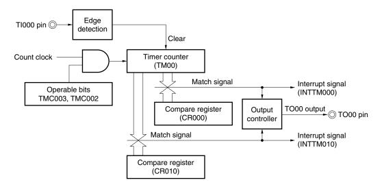
Figure 6-24. Timing Example of Clear & Start Mode Entered by Tl000 Pin Valid Edge Input (CR000: Compare Register, CR010: Compare Register)
