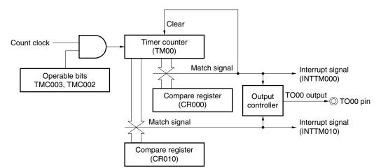
Figure 6-41. Block Diagram of PPG Output Operation
