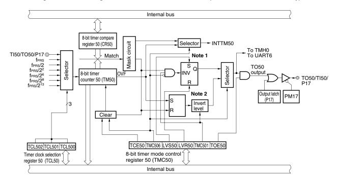
Figure 7-1. Block Diagram of 8-Bit Timer/Event Counter 50 (78K0/KB2-L, 78K0/KC2-L Only)
