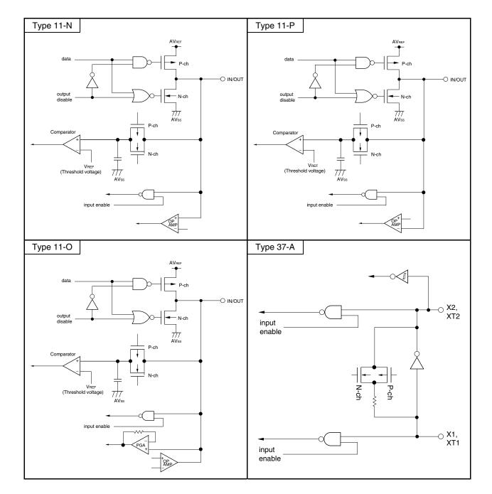
Figure 2-1. Pin I/O Circuit List (3/4)
