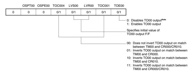
Note The timer output (TO00) cannot be used when detecting the valid edge of the Tl010 pin is used.
