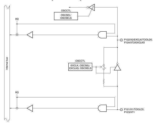
Figure 4-28. Block Diagram of P121 to P124
