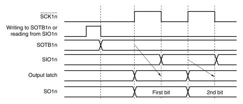
The first bit is directly latched by the SOTB1n register to the output latch at the falling (or rising) edge of  $\overline{SCK1n}$ , and output from the SO1n pin via an output selector. Then, the value of the SOTB1n register is transferred to the SIO1n register at the next rising (or falling) edge of  $\overline{SCK1n}$ , and shifted one bit. At the same time, the first bit of the receive data is stored in the SIO1n register via the SI1n pin.
