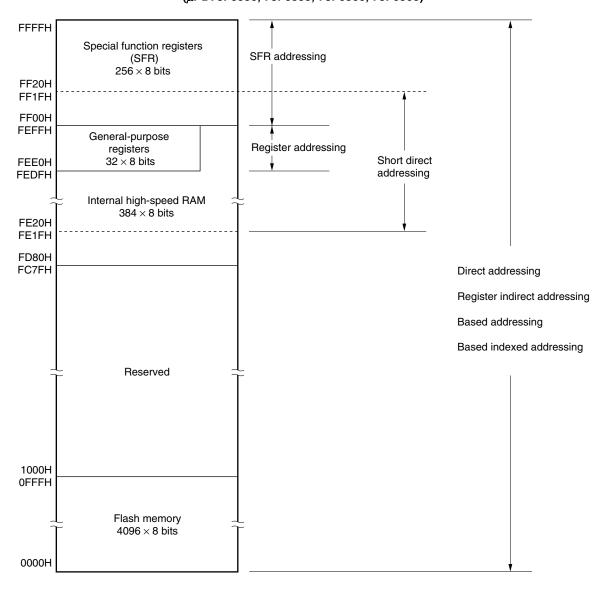
Figure 3-5. Correspondence Between Data Memory and Addressing  $(\mu PD78F0550, 78F0555, 78F0560, 78F0565)$
