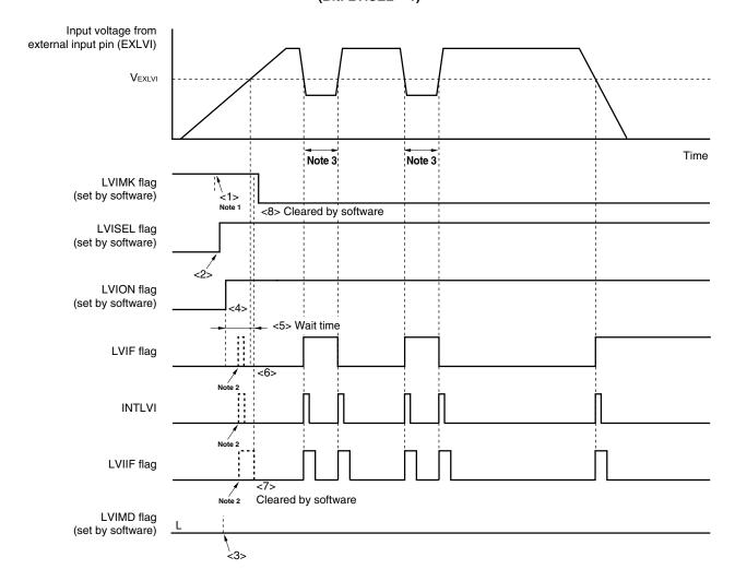
Figure 22-10. Timing of Low-Voltage Detector Interrupt Signal Generation
