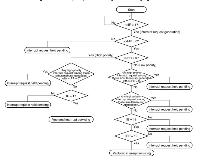
Figure 17-25. Interrupt Request Acknowledgment Processing Algorithm
