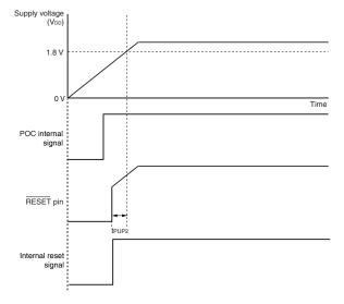
(7) LVI  $(T_A = -40 \text{ to } +85^{\circ}\text{C}, V_{PDR} \le V_{DD} \le 5.5 \text{ V}, V_{SS} = 0 \text{ V})$
