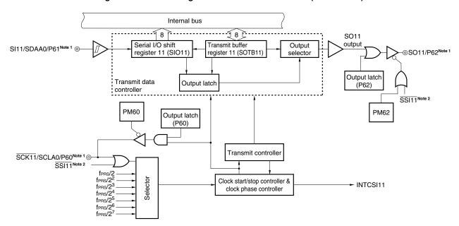
Figure 16-2. Block Diagram of Serial Interface CSI11 (78K0/KC2-L)
