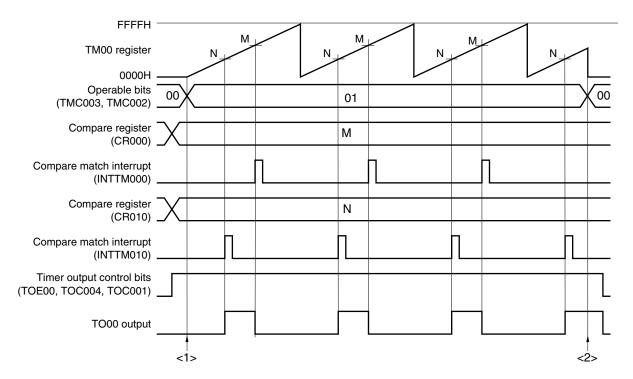
Figure 6-40. Example of Software Processing in Free-Running Timer Mode
