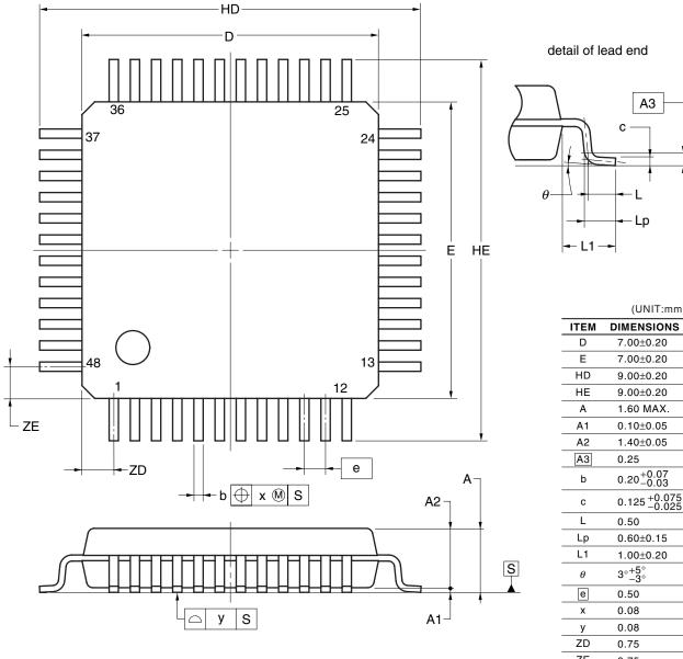
NOTE Each lead centerline is located within 0.08 mm of its true position at maximum material condition.
