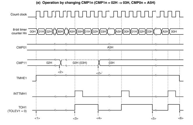
Figure 8-15. Operation Timing in PWM Output Mode (4/4)
