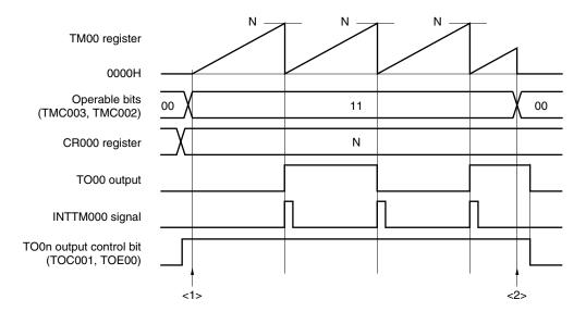
Figure 6-19. Example of Software Processing for Square-Wave Output Function
