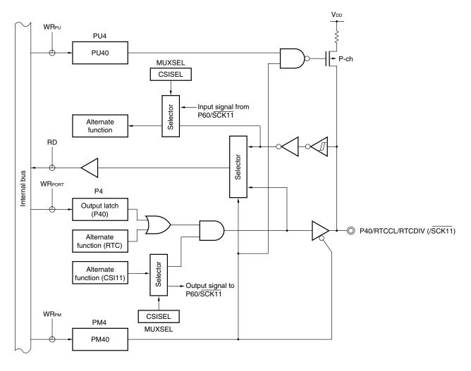
Figure 4-19. Block Diagram of P40
