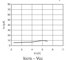
$T_A = +25$  °C,  $F_{MP} = 2, 4, 8, 10, 16$  MHz (divided by 2) Time-base timer mode with the external clock operating
