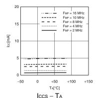
Vcc = 5.5 V, Fmp = 2, 4, 8, 10, 16 MHz (divided by 2) Main sleep mode with the external clock operating
