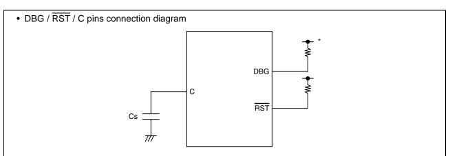
\*: Connect the DBG pin to an external pull-up resistor of  $2 \text{ k}\Omega$  or above. After power-on, ensure that the DBG pin does not stay at "L" level until the reset output is released. The DBG pin becomes a communication pin in debug mode. Since the actual pull-up resistance depends on the tool used and the interconnection length, refer to the tool document when selecting a pull-up resistor.
