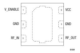
Figure 2. SKY65405-21 Pinout (Top View)
