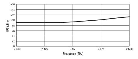
Figure 5. IIP3 vs Frequency
