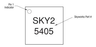
Figure 8. Typical Part Markings
