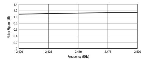
**Figure 4. Noise Figure vs Frequency**
