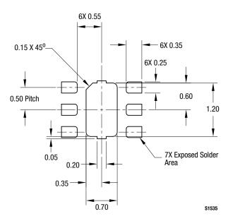
Figure 7. SKY65405-21 PCB Layout Footprint (Top View)
