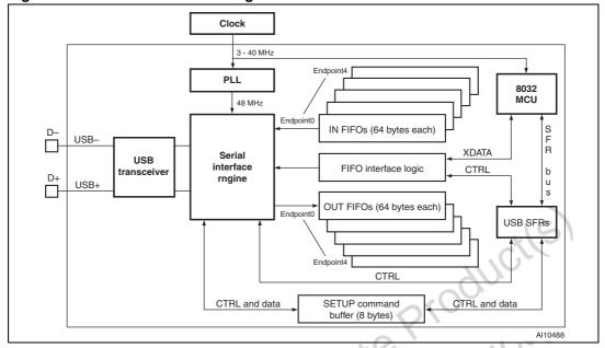
Figure 48. USB module block diagram
