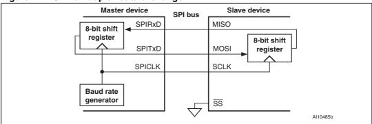
Figure 45. SPI receive operation example
