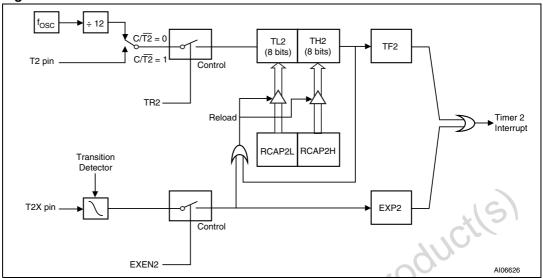
Figure 29. Timer 2 in baud rate generator mode
