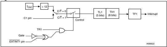
Figure 25. Timer/counter mode 2: 8-bit Auto-reload
