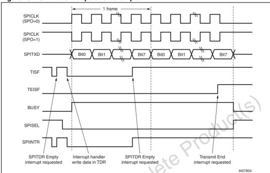
Figure 46. SPI transmit operation example
