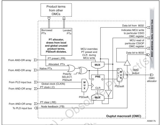
Figure 76. Detail of a single OMC
