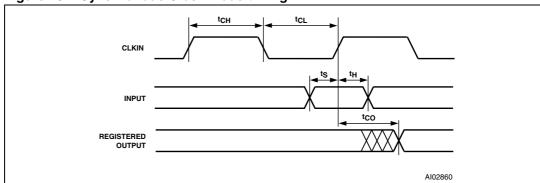
Figure 101. Synchronous Clock mode timing - PLD
