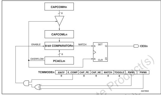
Figure 59. PWM mode - (x8), fixed frequency
