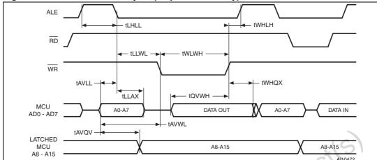
Figure 99. External WRITE cycle (80-pin device only)
