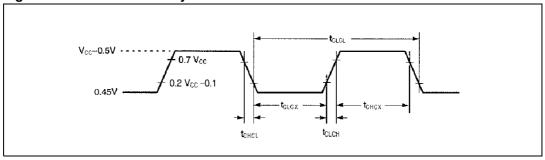
Figure 111. PSD module AC measurement I/O waveform
