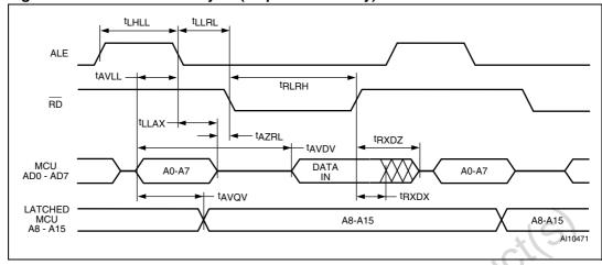
Figure 98. External READ cycle (80-pin device only)
