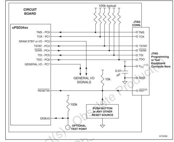
Figure 92. Recommended 6-pin JTAG connections
