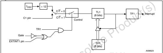
Figure 26. Timer/counter mode 3: two 8-bit counters
