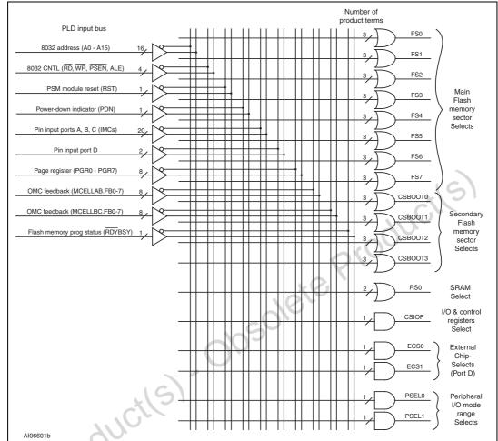
Figure 74. DPLD logic array
