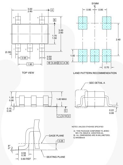
Figure 7. 5-Lead SOT23, JEDEC MO-178 1.6mm
