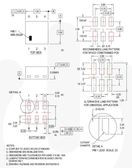
Figure 10.6-Lead, MicroPak2, 1x1mm Body, .35mm Pitch
