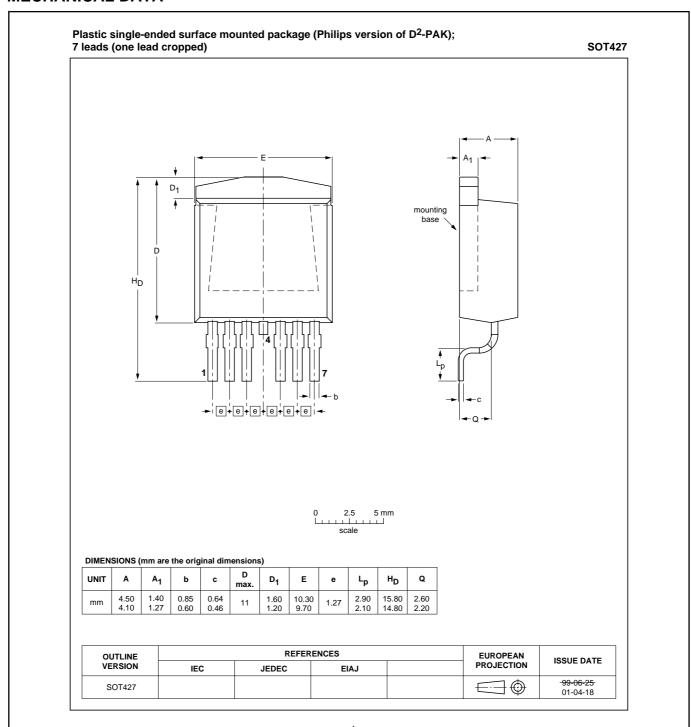
Fig.4. SOT427 surface mounting package<sup>1</sup>, centre pin connected to mounting base.
