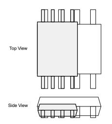
Figure 1. An TSSOP-8 Package Next to a SOIC-8 Package with Views from Both Top and Side
