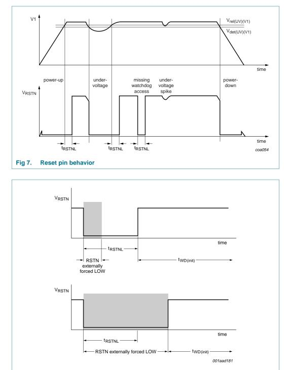
Fig 8. Reset timing diagram
