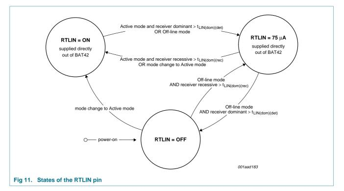
During Active mode, with no short-circuit between the LIN-bus and GND, pin RTLIN provides an internal switch to BAT42. For master and slave operation an external resistor, 1 k $\Omega$  or 30 k $\Omega$  respectively, can be applied between pins RTLIN and LIN. An external diode in series with the termination resistor is not required due to the incorporated internal diode.
