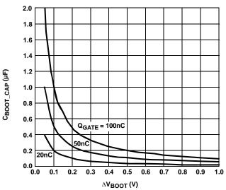
FIGURE 2. BOOTSTRAP CAPACITANCE vs BOOT RIPPLE **VOLTAGE**
