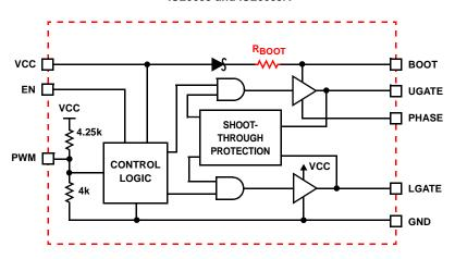
INTEGRATED  $3\Omega$  RESISTOR (RBOOT) AVAILABLE ONLY IN ISL6609A
