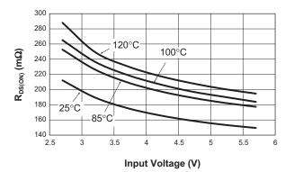
N-Channel  $R_{DS(ON)}$  vs. Input Voltage
