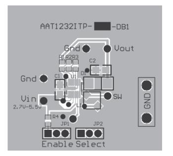
Figure 4: AAT1232 Evaluation Board Top Side Layout.
