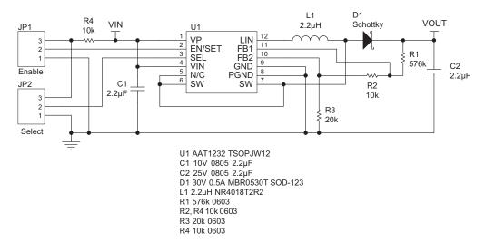
Figure 1: AAT1232 Demo Board Schematic.
