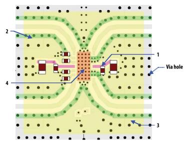
Figure 4. PCB guideline on phone board
