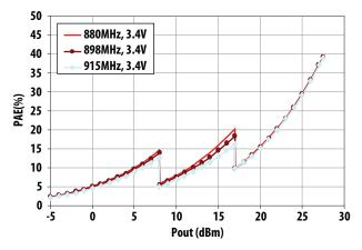
**Power Added Efficiency vs. Output Power**
