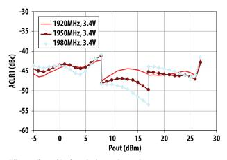
Adjacent Channel Leakage Ratio 1 vs. Output Power
