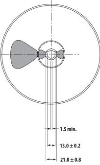
Plastic Reel Format (all dimensions are in millimeters)
