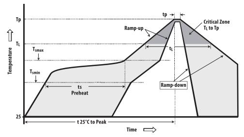
Typical SMT Reflow Profile for Maximum Temperature =  $260 + 0/-5^{\circ}C$
