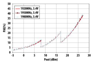
Power Added Efficiency vs. Output Power
