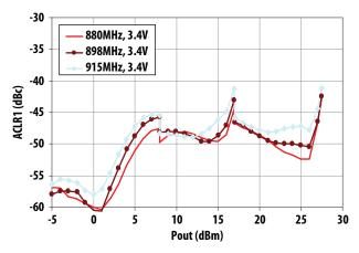
Adjacent Channel Power Ratio 1 vs. Output Power
