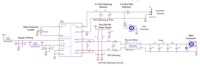
Figure 4.1. Schematic of the RF Section of the BRD4258A
