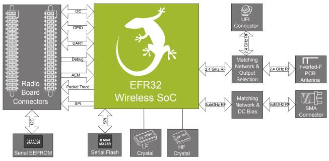
Figure 3.1. BRD4258A Block Diagram
