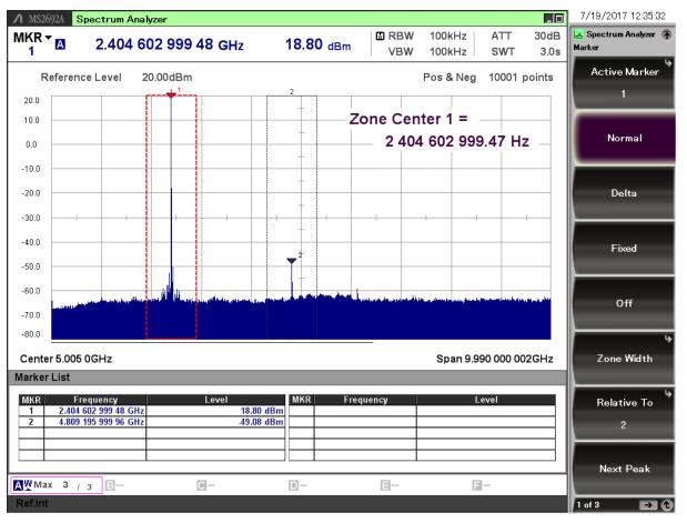
Figure 7.2. Typical Output Spectrum of the BRD4258A
