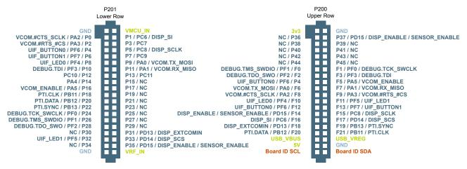
Figure 2.1. BRD4258A Radio Board Connector Pin Mapping
