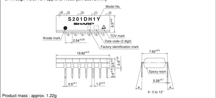
(Note) To radiate the heat, solder the lead pins ④ to ⑦, ⑨ on the pattern of the PCB without using a socket such that there is no open pin left. (Unit : mm)
