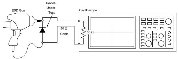
Figure 4. Diagram of ESD Test Setup
