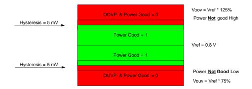
Figure 22. OOV and OUV Window Diagram
