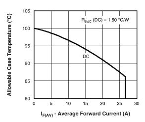
Fig. 5 - Maximum Allowable Case Temperature vs.
