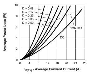
Fig. 6 - Forward Power Loss Characteristics
