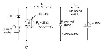
Fig. 8 - Unclamped Inductive Test Circuit
