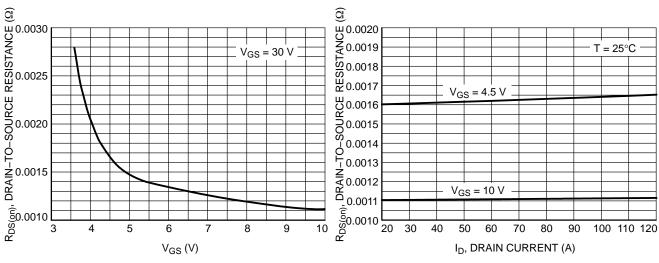
Figure 3. On-Resistance vs. V<sub>GS</sub>
