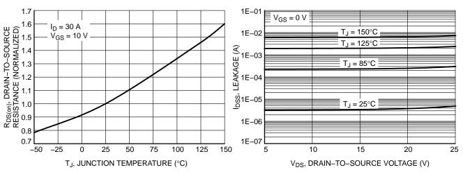
Figure 5. On-Resistance Variation with **Temperature**
