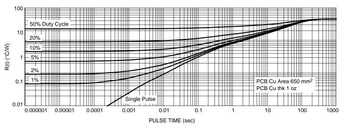
Figure 13. Thermal Characteristics
