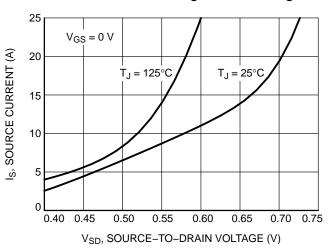
Figure 10. Diode Forward Voltage vs. Current
