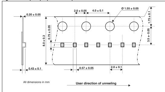
Figure 12. Flip Chip tape and reel specification
